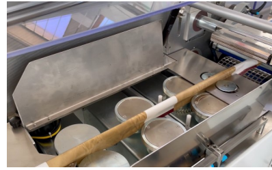
Three (3) pairs of sealing rollers, 1st one inclinable
