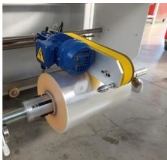
Motorized film unwind
